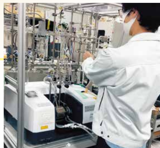
Molecules adsorbed on the electrode surface are observed with infrared light
