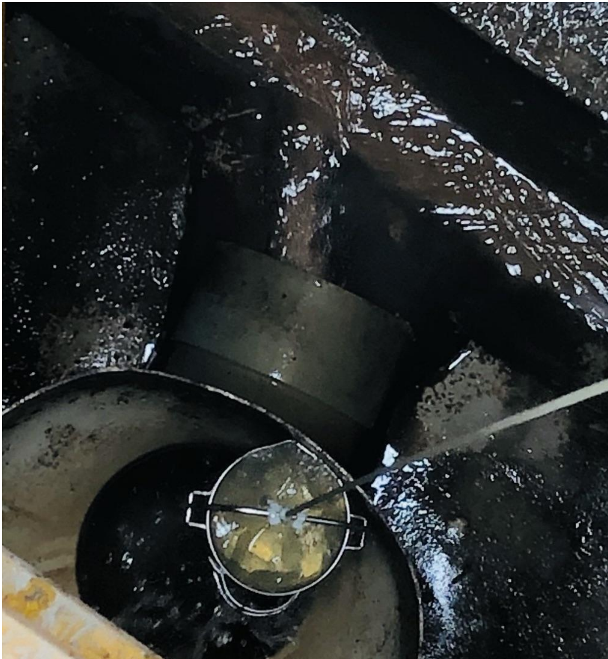
Wastewater sample being collected from a manhole in the village (Photo: Masaaki Kitajima).
