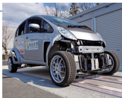
An electric vehicle utilizing dynamic wireless power transfer from coils buried in the road to the vehicle's in-wheel motor.
