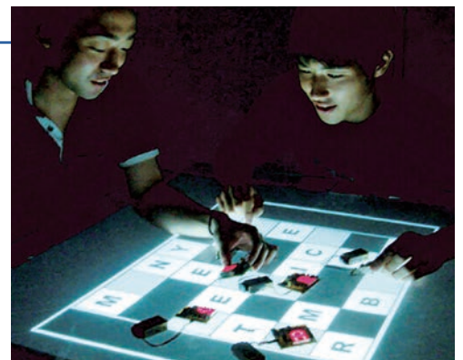
"EmiTable", a table-type display that reveals hidden light signals as visible pixel units.
