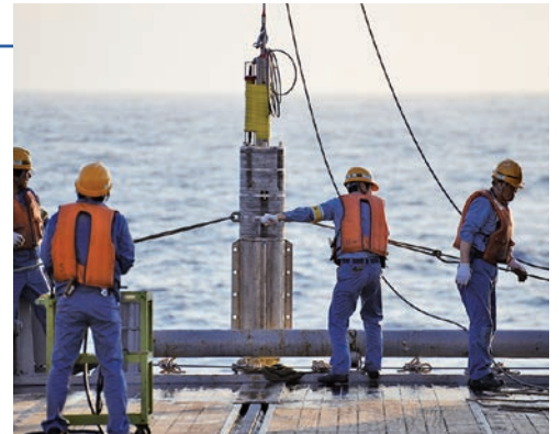
Survey on rare-earth elements and yttrium (REY)-rich mud conducted near Minamitorishima Island using a piston corer
