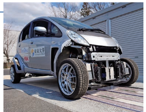
An electric vehicle utilizing dynamic wireless power transfer from coils buried in the road to the vehicle's in-wheel motor.
