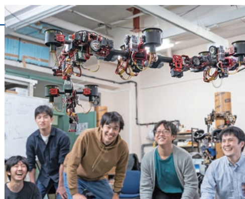
Fully-transformation-type multi-linked flying robot
