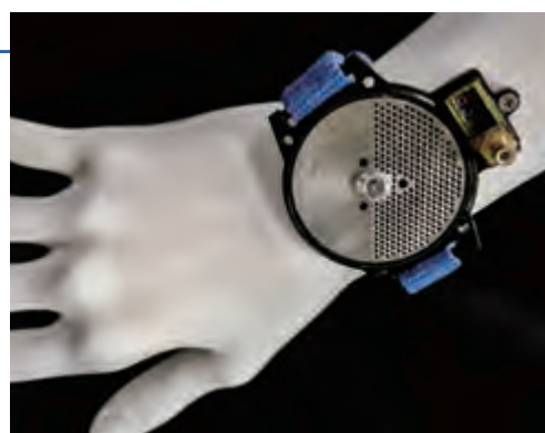
Electret device generating electricity from arm movement
