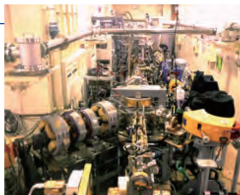
LINAC facility where ultra short pulse electron beams are generated
