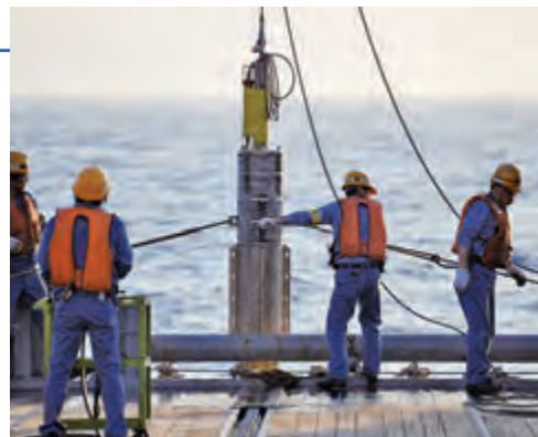
Survey on rare-earth elements and yttrium (REY)-rich mud conducted near Minamitorishima Island using a piston corer
